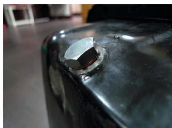
4. Place a washer on new oil drain nut and install the new one into renewed hole.
