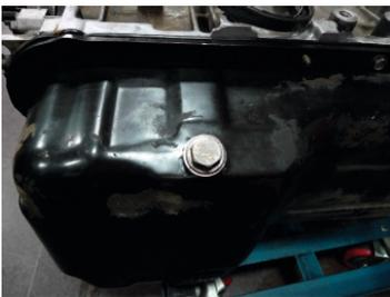
1. Disassemble the damaged oil drain screw.
